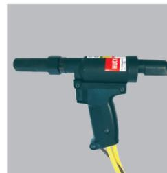
Hydraulic installation with extra long stroke. Ideal for installing 9.5mm Magna-Lok® and 7.9 mm Floortight®. Will also install 7.9 and 9.5mm Lockbolts & structural blind rivets.
