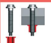
**Unique helical lock groove (upwards from 9.5mm):** Holds pins and collar in place prior to installation\*
