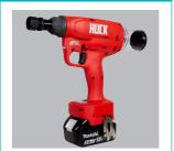
Battery powered installation too with electronically adjustable pull force control. Installs structural blind rivets and LockBolts up to 6.4mm.
