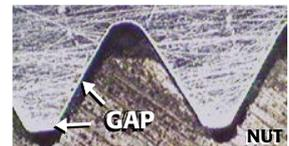
Regular nuts and bolts have a gap, which allows for loosening by vibration.
