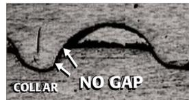
The swaged collar forms over the lock thread, and eliminated the gap.
