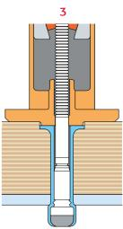
Continued pulling on the pintail forms a mechanical lock between the pin and sleeve end. The anvil on the installation tool then countersinks the fastener head into the top of the material to a preset depth set by the anvil. The anvil's large bearing face then prevents further travel of the sleeve head into the top material.
