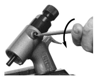
5. Remove Pull Piston 15 from the tool head by inserting a small punch into the front of the Piston and tapping gently with a hammer.
