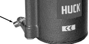
5. Set air supply pressure regulator to 6.2-6.9 bar (90-100 psi). Connect air hose to tool.
