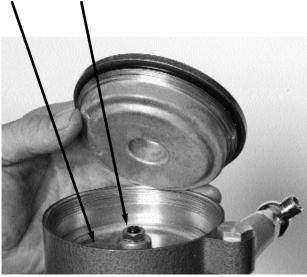
12. Use a pair of locking pliers, (eg. Mole Grips), locked onto the Nut 61 and pull the Air Piston assembly out of the cylinder.
