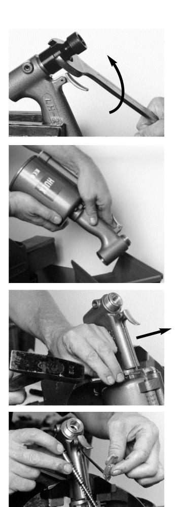
11. Clamp inverted tool finally in a vice, (use fibre vice clamps). Use a 28 mm socket wrench to unscrew Cylinder Cap 51 anti-clockwise and expose Air Piston 58 & Nut 61.
