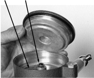
2. Use a pair of locking pliers, (eg. Mole Grips), locked onto the Nut 61 and pull the Air Piston assembly out of the Air Cylinder.
