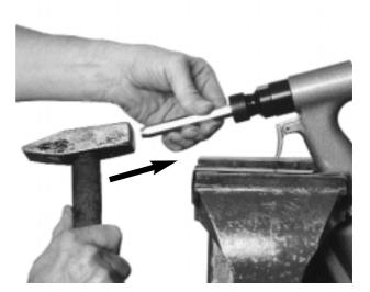
The Piston will slide out and can be removed.
