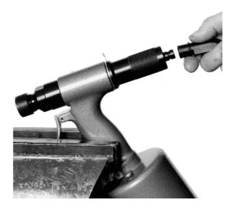
2 Finnly hold the Handle of the Installation Tool in a vice, (use number faced vice grips). Remove Deflector. Unscrew the Rear Gland 21 from the head of the tool.
