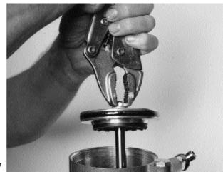
5. Clamp inverted tool firmly in a vice, (use fibre vice clamps). Apply a thin coating of grease to the O Ring 53 on the Cylinder Cap 51. Use a 28 mm socket and torque wrench to tighten the Cylinder Cap 51 clockwise into the Air Cylinder. Tighten to 25 to 30 Ft.1b (33.90 to 40.68 Nm).
