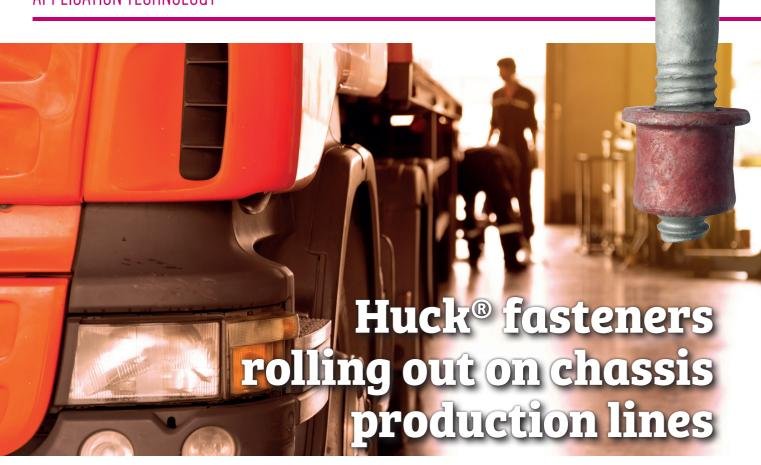
Star Fasteners has recently helped truck and trailer body builders to eliminate the need for any welding in the construction of the subframe of a chassis, thanks to the use of Huck® BobTail® fasteners.
