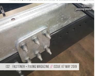
arranged a demonstration where I went over to Ireland with the tooling and the fixings to show how the BobTail would work in the application. The customer could see with their own eyes how quick and easily the BobTail installed, as well as its strength capabilities, and they decided to change from welding to using the BobTail."
