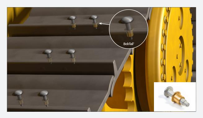
High-strength, fast and easy installation, along with unmatched vibration resistance are what make HuckBolts\* the smart choice for heavy equipment assembly applications, whether for agriculture, mining, or construction.
