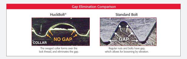
When compared with conventional nuts and bolts, HuckBolts have a much larger cross-sectional area and larger root radius, resulting in a much stronger and more secure joint. In fact, HuckBolts have up to 30% more bolt cross-sectional area, and up to 5x larger root radius than regular bolts, depending on the bolts used.
