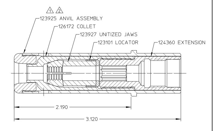
NOTE: THIS NOSE ASSY IS TO BE USED WITH POSITIVE EJECTION TOOLS ONLY
