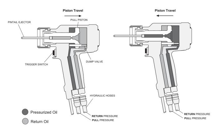
Pull Pressure (Pull Cycle) Fig. 1(a)
